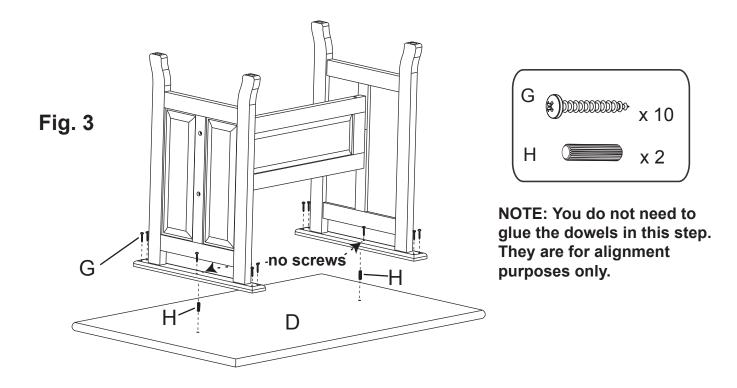
**3.** Place Top (D) face-down on a clean, protected surface. Insert two Dowels (H) into the dowel holes as shown in Figure 3. Position the leg assembly so that the corresponding dowel holes in the top supports fit over the dowels in the seat. Using the predrilled holes in the Top Support as guides, secure with #8x1½ Pan Head Screws (G). See Figure 3.
