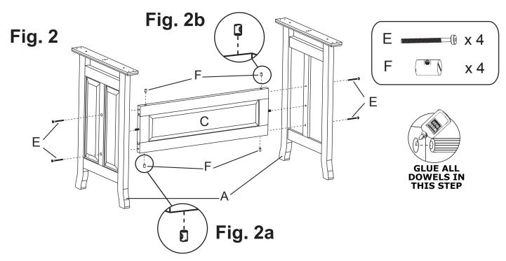
2. Spread a thin film of glue in the dowel holes on the Legs (A). Insert Middle Support (C) and quickly wipe away any excess glue. See Figure 2.
