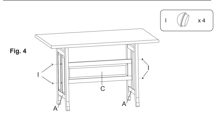
**4.** Glue Wood Buttons (I) into the exposed holes. Wipe away any excess glue. See Figure 4. Adjust the Glides (M) in the bottoms of the legs to level your table.
