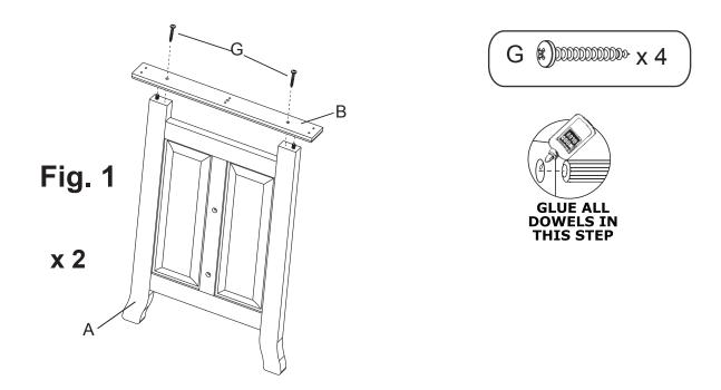
1. Spread a thin film of glue into the dowel holes of the Top Support (B) and place over dowels of the Leg (A). Gently tap with a padded hammer and quickly wipe away any excess glue. Secure with #8x11/4" Pan Head Screw (G). See Figure 1.
